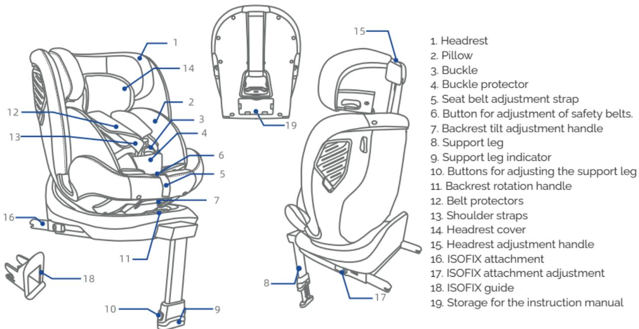
Check the product for missing components. Contact your dealer for missing or damaged components.
